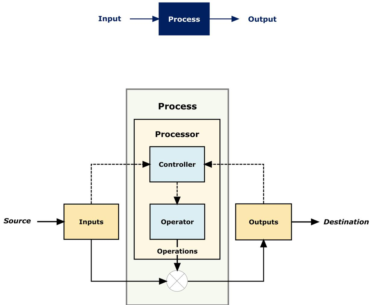
It is common enough to see the basic input-process-output graphic as shown at the top of this page. But, have you ever wondered what's inside that process box? The diagram immediately above sheds some light on that. What's inside is a processor, interacting with the inputs. And inside the processor is an operator, carrying out the operations that define the process, and a controller riding herd on everything. For more about what's inside the process box, click [here](#).
